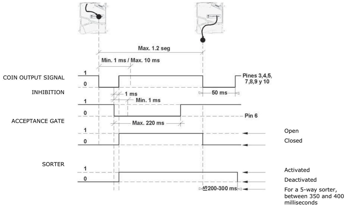
The second picture shows the instant when the coin has passed all the sensors that are used for its analysis and the validator starts its communication with the machine
