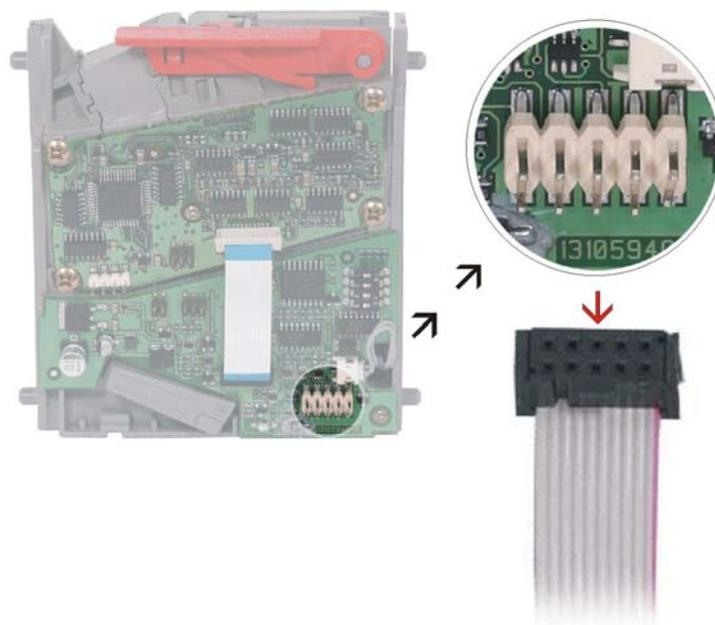
2nd. Remove the cover of the *validator* and activate *Dipswitch 1* to determine the number of the coin or token you wish to programme.
