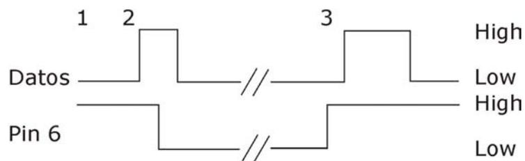
**FIGURE 1:** A valid coin has been detected
