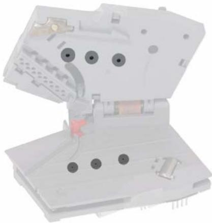
3 pairs of infrared sensors that obtain parameters related to the diameter of the coin.
