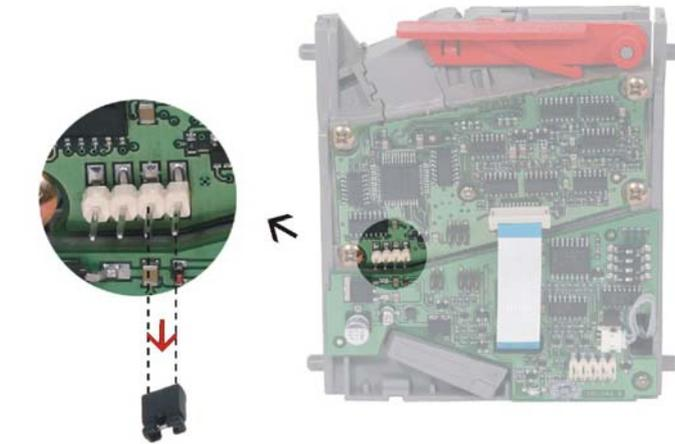
To eliminate the coin or token programmed: place and then remove the short on pins 1 and 2 of the 4-way connector J5
