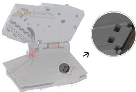
In the lower part of the entry model is the acoustic sensor. This device receives the sound made by the coin when it hits the *metallic cylinder* on falling into the validator. The parameters received by this sensor are very important in the coin acceptance or rejection process.
